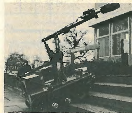
Not quite the shape of things to come as foreseen by H. G. Wells or Isaac Asimov, but a working robot called Commander Bill. Developed by the Research Group at Warwick University, the robot has been specially designed to operate over rough terrain and to negotiate steps.
